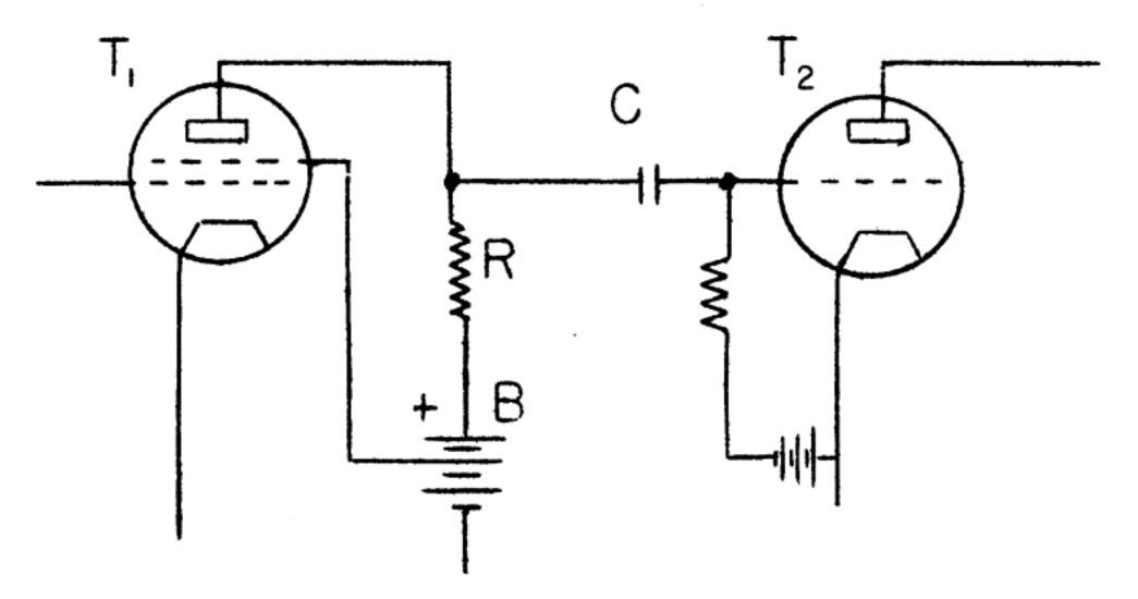
The above figure represents a conventional stage of resistance coupling. The gain for this stage is the product of the resistance, R, multiplied by the Mutual Conductance in mhos of the tube  $T_1$ . Suppose R is 100,000 ohms and the mutual conductance of  $T_1$  is 750 micromhos, then:
