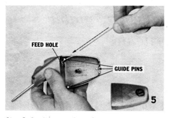
Step 3. Straighten at least 2 inches of the end of the solder. (Bends, kinks, or hooks on the end will make loading difficult, figure 5). Line up straight end of solder in feed hole (arrow) so that it points straight through the center of the probe, and insert about 2 inches of solder into the action until a
