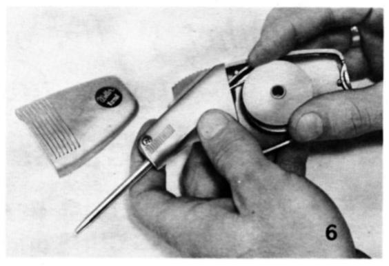
slight resistance is felt. Place spool on hub (figure 6) and operate ribbed actuator until solder appears at end of probe. Replace cover by lining up three guide pins (see figure 5) and snapping cover firmly in place. Now, you're ready to solder!
