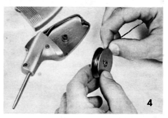
solder clean). Difficulties in feeding solder, and in solder wedging tight on the spool will be eliminated completely with a few seconds extra care in winding the spoon evenly. **Note:** Although the Weller Kormat will handle solder ranging from 22 gauge (.028 inch Dia.) to 15 gauge (.072 inch Dia.), best results are with 18 or 19 gauge (.040 to .050 inch Dia.)
