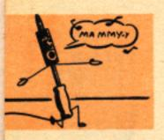
DO disconnect iron when not in use so that flux won't burn out and blacken copper. Oxidation insulates the tip and the iron will not solder efficiently.
