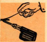
DON'T try to solder by applying heat to the solder itself.
