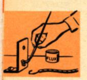
DO apply flux only to the part being soldered. Be especially careful to keep it away from threads of any screw-type iron.
