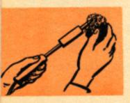
DON'T permit oxidation to remain if iron becomes overheated—and DON'T use a file on it unless tip is pitted.
