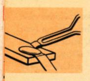
DO slide the tip from your work. This gives an even soldered surface.
