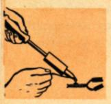
DON'T try to solder wire joints and similar work by holding the soldering tool above the work. DO hold the tip under the wire joint and solder above it, so that tip supports solder until it becomes hot enough to flow into joint.
