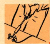
po have a heavy film of solder between the working face of the tip and the joint to be soldered. This conducts heat from the tip to the work.
