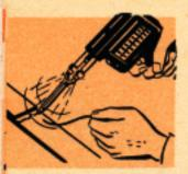
pre-tin by spreading solder over joints and surfaces with the hot tip. Work the solder into the surface with
