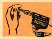
Wellertips are easy to keep tinned and bright; and they can be replaced easily and inexpensively if pitted or damaged.
