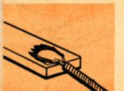
pon't allow acid flux to remain on work after soldering is completed. DO remove at once to avoid corrosion.
