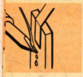
DON'T try to solder a vertical surface by applying solder with the tip of the iron.
