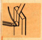
DO apply solder to the trough formed by the tip and the surface to be soldered — then press tip against the surface.
