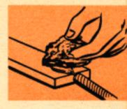
Remember that Rosin flux will not cause corrosion and need not be removed unless flaking will be harmful. Acid flux must be removed at once.
